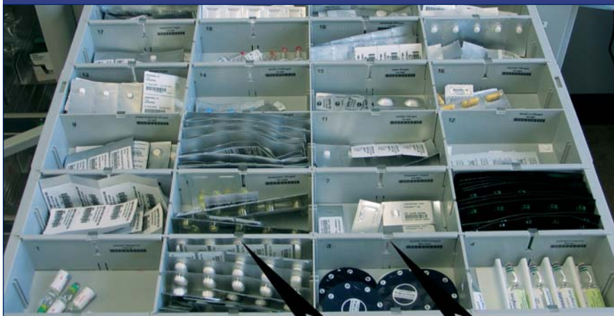
Figure 2: Matrix drawer equipped with a light-guided system (arrows indicate position of light-emitting diodes). Omnicell configuration, Department of Respiratory Medicine, OLVG Hospital
